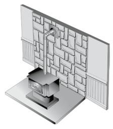
Pellet stoves are also available as fireplace inserts installed in masonry or factory-built metal fireplaces. Since PelletVent Pro is smaller in diameter than normal chimneys, it can be installed as a chimney liner. A 60" length of stainless flex permits installation through the existing fireplace damper.
