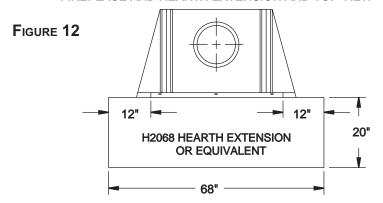
NOTE: A hearth extension placed on a combustible floor must be constructed with rigid insulation which has a minimum "R" value of 1.16 or a "K" value of 0.43. The insulation must be covered with a non-combustible covering such as a tile stone, marble, or a piece of 0.018 minimum sheet metal which is needed to protect the insulation. Follow instructions provided with the fireplace for all other specifications and directions for proper installation of the fireplace and hearth extension.
