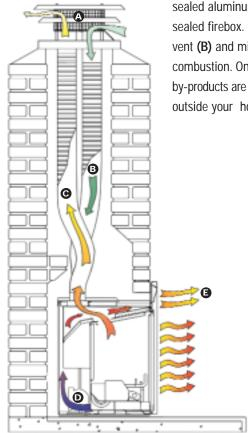
A balanced Flue Termination Cap (A) is installed at the top of your existing chimney and connected to the co-linear sealed aluminum venting that lead to The Broadway's sealed firebox. Outside air is then drawn through the intake vent (B) and mixed with natural or propane gas to create combustion. Once this process has taken place, combustion by-products are expelled through the exhaust vent (C) to outside your home.
