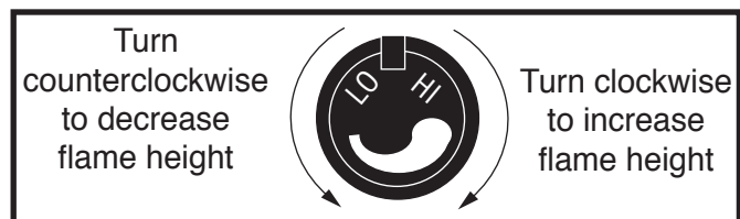
Fig. 49 Flame adjustment knob for Honeywell valve.
